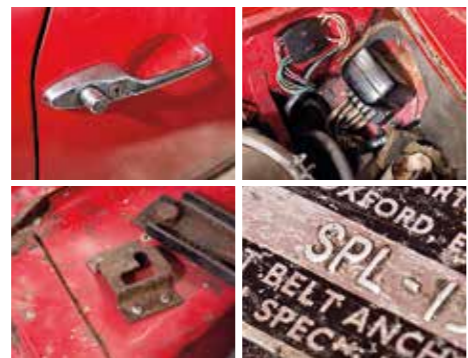
Further clues to the car's prototype origins include the Elf/Hornet door handles, the voltage regulator on a riveted plate on the bulkhead, the 'SPL' chassis tag and the '69' date on the wiper motor.
