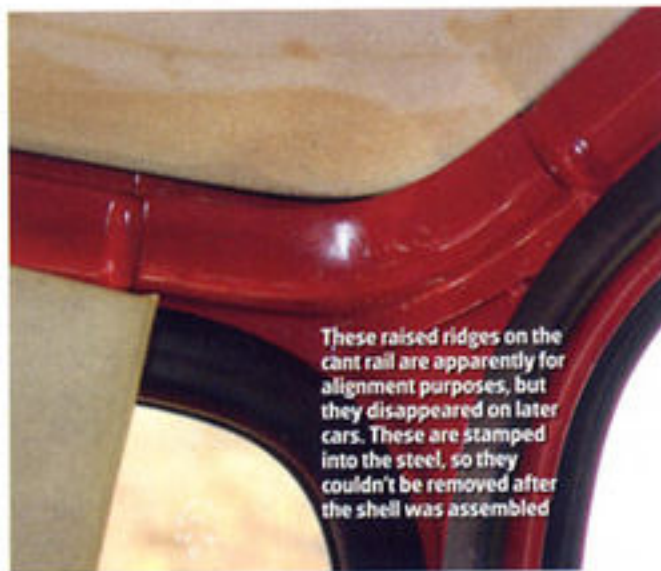
For a utilitarian vehicle, the Mini had lots of lights so passengers could see their oddments! And the heavy card liner is actually a full box that can be lifted out as one piece, which is something Simon hasn't seen before
