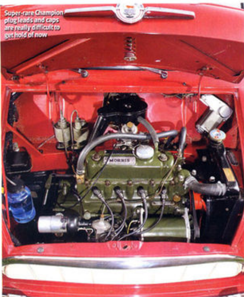
Carburetor is the original SU 1 1/2-inch, with its brass dashpot cap
